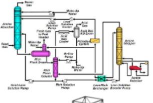
Raw natural gas streams often contain impurities that can cause significant damage to process, pipelines and equipment. Our acid gas removal solutions effectively remove hydrogen sulfide (H2S) and carbon dioxide (CO2) from gas streams to meet product specifications and protect downstream equipment.
